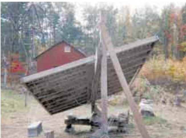
Detail of one of the home-built trackers. Notice the concrete block as counterbalance.
