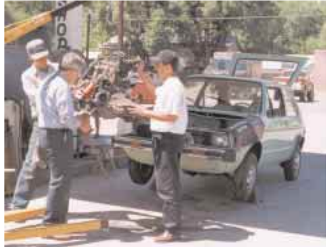
Hoisting out the internal combustion engine.
