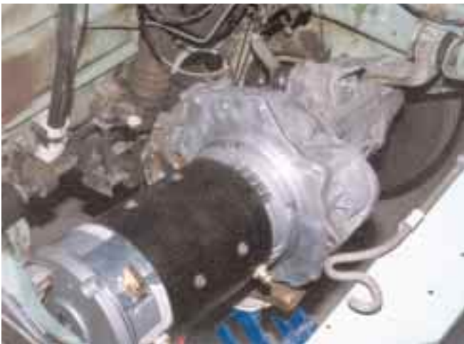
An aluminum and steel adaptor system mates the new electric motor to the standard transmission.
