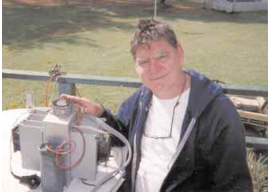
John with his home-built, 6 KW, 120 VDC in, 120 VAC out square wave inverter. It draws 3 watts at idle and is 99.5 percent efficient with a 1,000 watt load.
