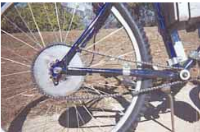
Drivetrain from the 13 tooth sprocket on the bottom bracket spindle to the 60 tooth sprocket on the rear hub.
