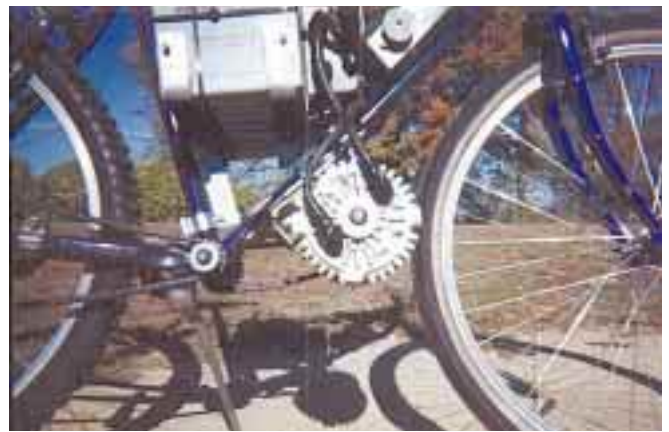
The Scott Motors 24 VDC PM motor and two PowerSonic 28 AH batteries can drive this bike to 30 mph.
