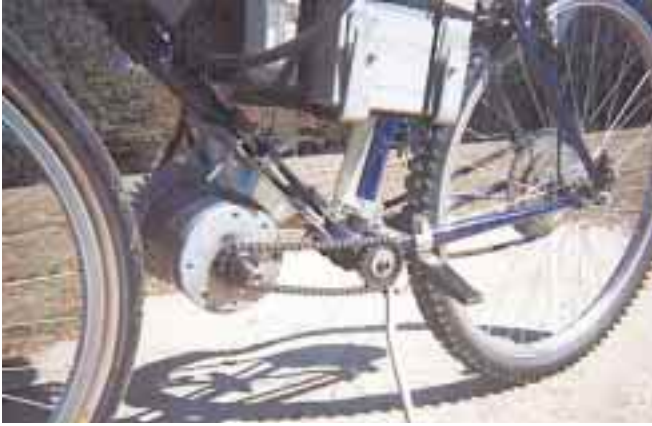
Drivetrain from the 1 hp motor to a 20 tooth sprocket on the bottom bracket spindle.
